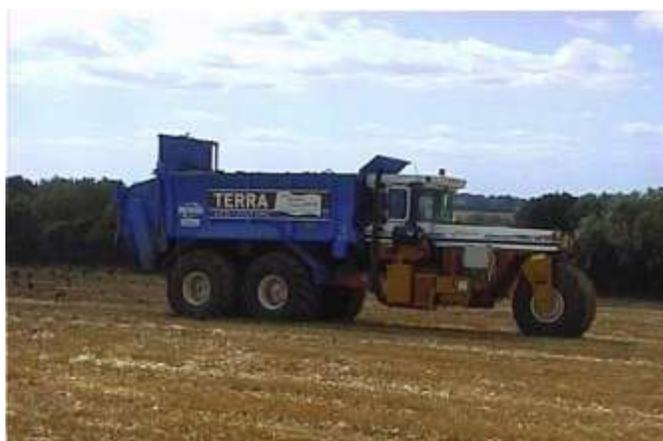
**Figure 2 Biosolids application equipment**
