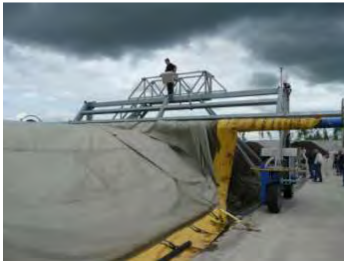
Figure 5 Gore windrow cover deployment and retrieval machine at Moncton, NB, CA - the cover is tied down to limit windlift when the water ballast tubes have been drained.
