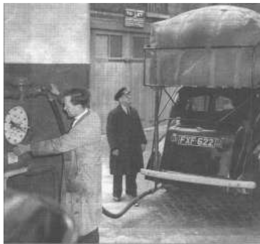
Figure 2 Using biogas as road fuel around 1943 - the idea is not new but the implementation has improved
